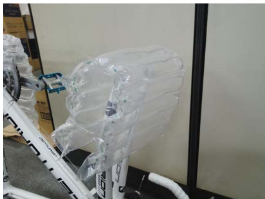
Put the padding around front fork
