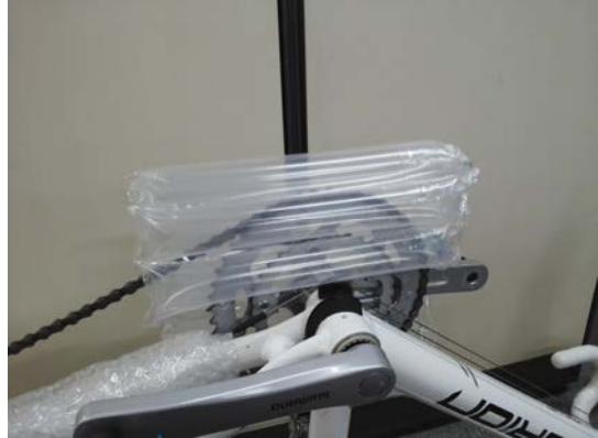
Put the padding around chain ring
